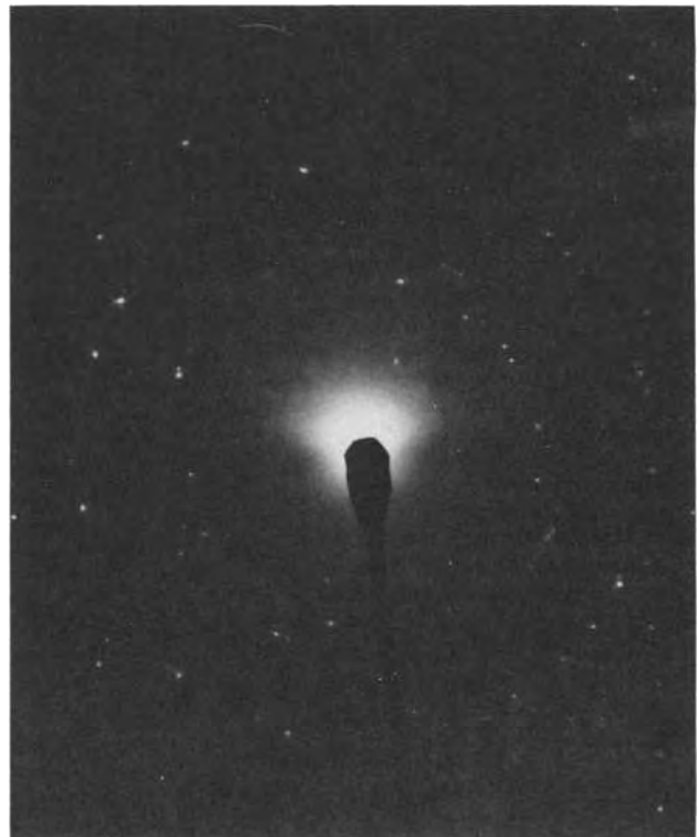
Fig. 2. Reflection electron diffraction pattern of a boron arsenide film deposited on the silicon face of a hexagonal silicon carbide substrate at 850°C.
