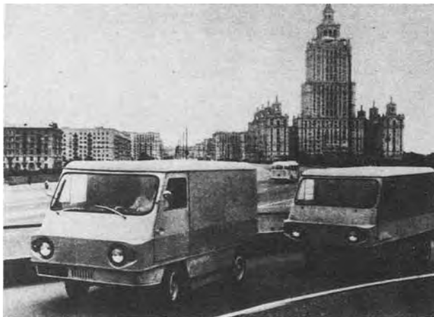
Fig. 12. Soviet prototype electric van EM-0466. Motors, two d.c.; range, 48 miles; speed, 27 mph; weight, 1700 kg; load capacity, 454 kg.
