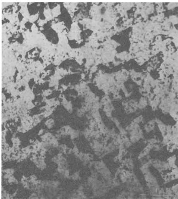
Fig. 3. Electron micrograph of oxidized film (700°C, 2 \times 10^{-7} Torr, 15 min). FeO grains are randomly distributed.
