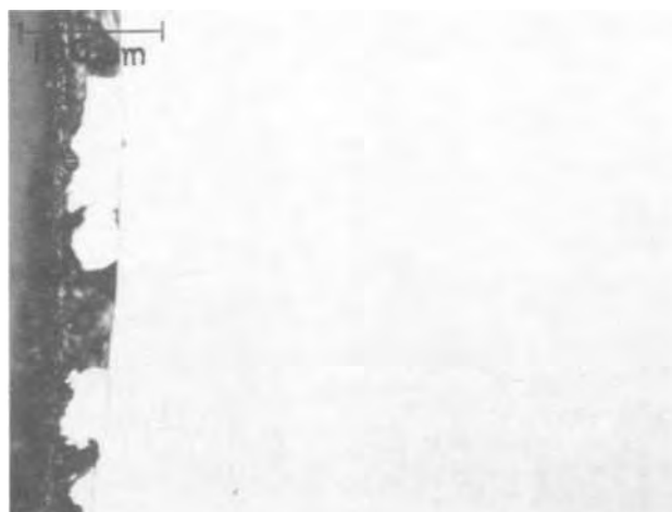
Fig. 3. Inclusions in InAs layer grown at 650°C. Layer thickness 2 \mu\text{m} .
