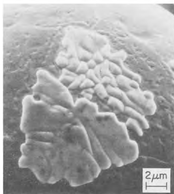
Fig. 12. Location of pits with respect to receding silver chloride deposit. a (left), SEM photograph; b (right), graphical representation
