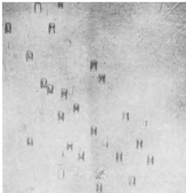
Fig. 1 (a). Etch pits produced on the (001) face of the Gd 2 (MoO 4 ) 3 by 40% HNO 3 (45 sec of etching time). This face developed the positive electrostatic charge on heating ( \times 400 ).
