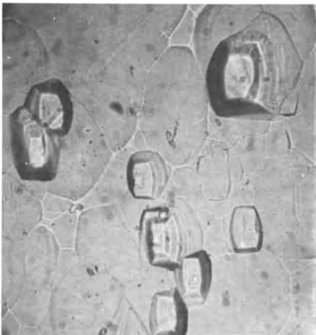
Fig. 3. Pits produced on (001) c-face by 25% water solution of HCl, with 15 sec of etching time ( \times 400 ).
