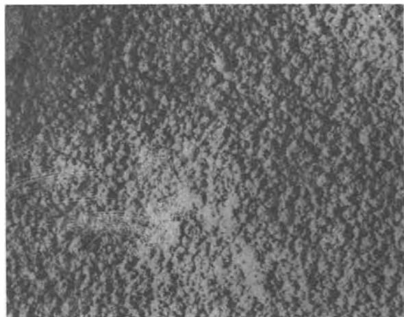
Fig. 15. ECRC's electrodeposition of zinc on the anode at 600 A/m 2 .
