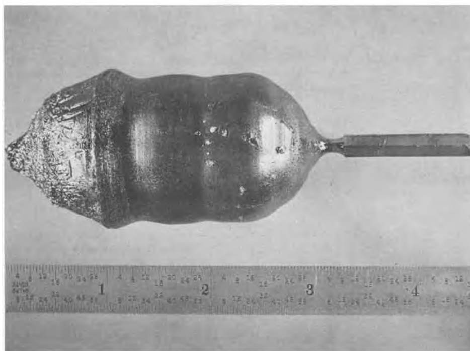
Fig. 7. Photograph of a crystal typical of those which can be grown by means of the x-ray imaging system.
