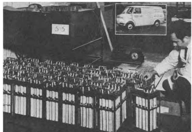
Fig. 21. British Railway's and ECRC's 30 kW sodium-sulfur powered delivery van.
