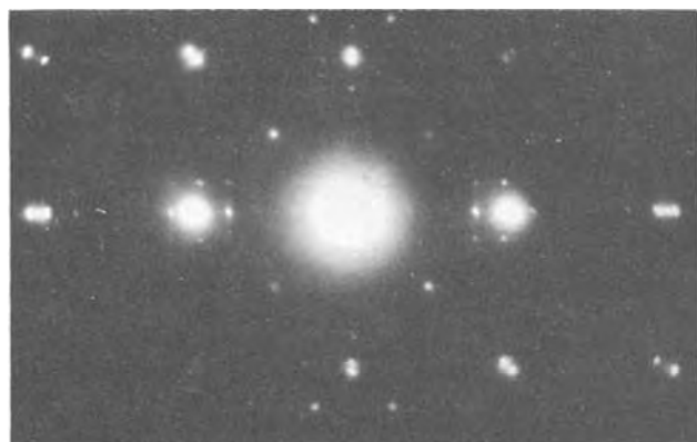
Fig. 2. Diffraction pattern of oxidized film ( 700^\circ\text{C} , 2 \times 10^{-7} Torr, 240 min). Four phases show: Fe, FeO, \text{Fe}_3\text{O}_4 , \text{Fe}_4\text{N} .
