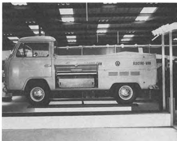
Fig. 2. Volkswagen electric van showing battery rack. Battery type, lead-acid; maximum range, 60 miles; maximum speed, 45 mph; payload, 2000 lb.
