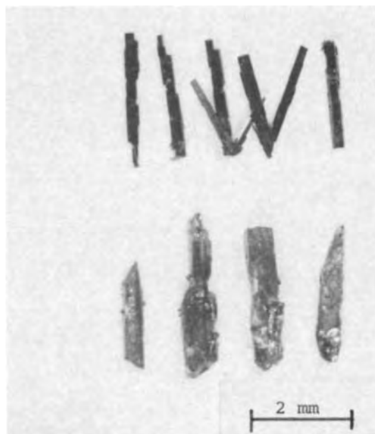
Fig. 2. Gallium nitride crystals grown on the wall of the silica tube (upper) and in the alumina boat (lower) by the sublimation technique.
