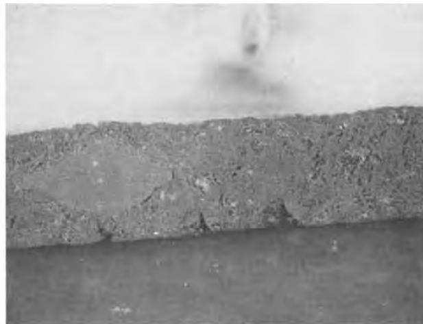
Fig. 4. The appearance of a cross section of a negative plate containing no lignin but 0.5% BaSO 4 after 27 cycles. Compare thickness of plate with that of Fig. 5. Magnification 17 \times . Plate is charged.
