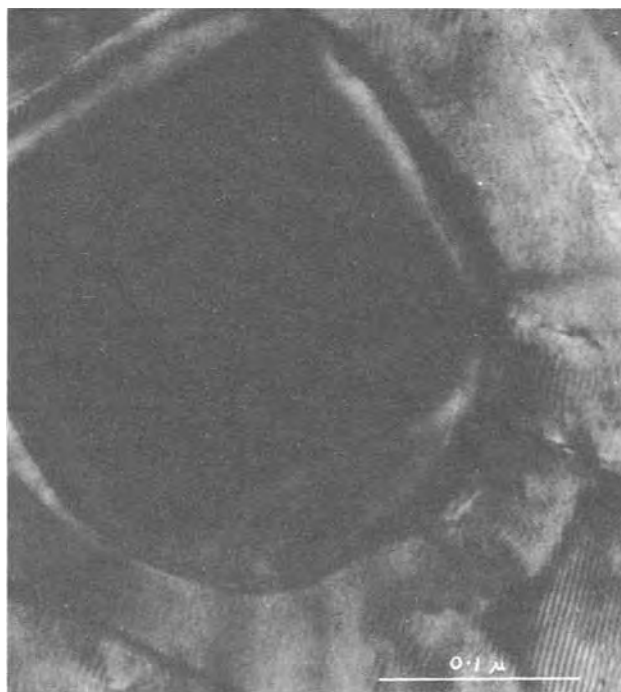
Fig. 6. Electron micrograph of oxidized film (700°C, 2 \times 10^{-7} Torr, 240 min). At high resolution three distinct sets of moire fringes appear.
