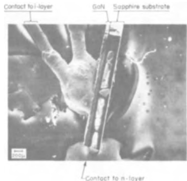
Fig. 6. Perpendicular view of diodes as seen in the scanning electron microscope. The entire device (including the sapphire substrate) and the two metal contacts (to the n- and i-layers) are visible. Magnification 25 \times .
