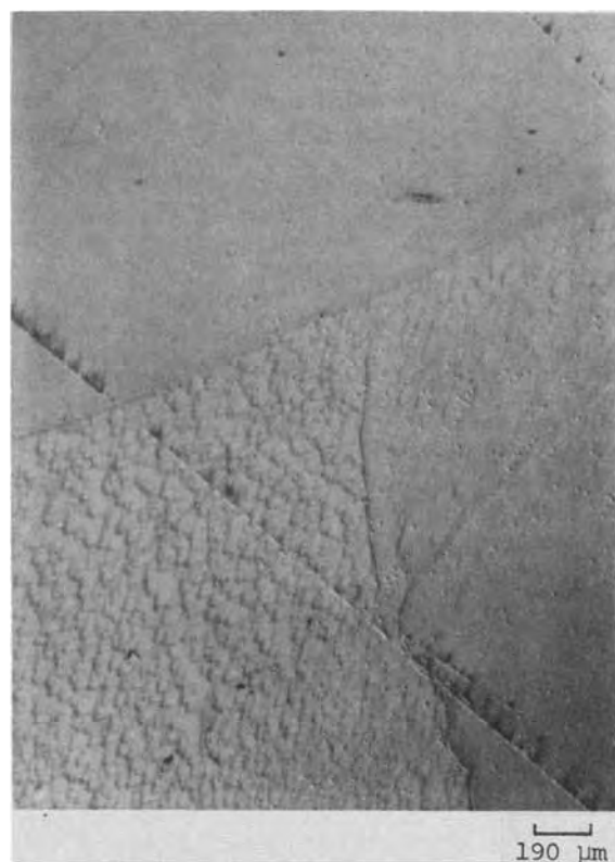
Fig. 4. Defects in Verneuil (01 \bar{1} 2) \text{Al}_2\text{O}_3 revealed by etch-polishing with Freon-13 (about 8 \mu\text{m} removed).
