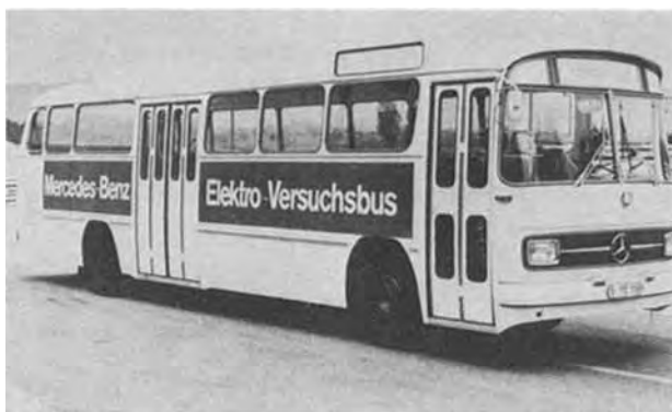
Fig. 4. Mercedes hybrid-electric bus. Battery type, lead-acid; rating, 380V, 275 A-hr; maximum range, 180 miles; maximum speed, 35 mph.
