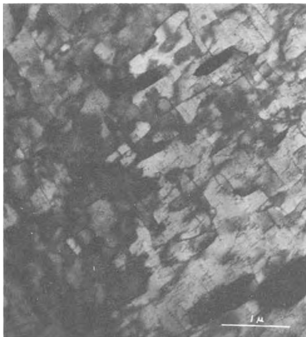
Fig. 1. Electron micrograph of grid-annealed film. Low angle grain boundaries are marked by piled-up dislocations.
