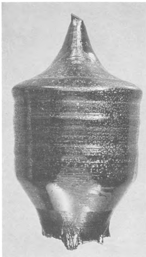
Fig. 8. Photograph of crystal whose diameter of 1.56 in. was controlled to within 20 mils.
