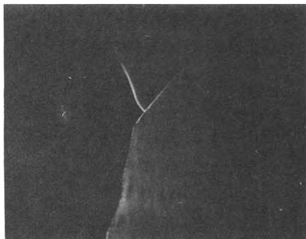
Fig. 5. Microscopic photograph (32 \times ) of a fracture illuminated by polarized light and viewed through a polarizer (analyzer).
