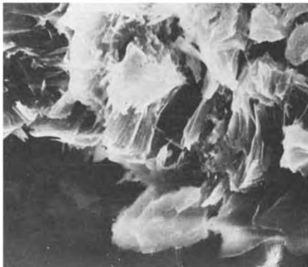
Fig. 7. Be electrode surface after polarization in 0.2M KCl/aq. Magnification 800X.
