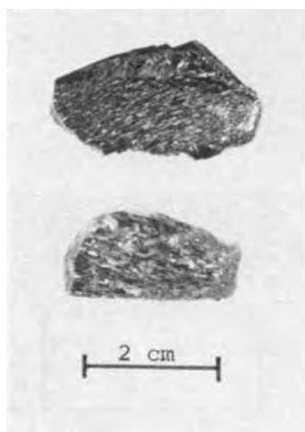
Fig. 6. Gallium nitride crystals obtained by the ammonolysis of gallium monochloride. The upper crystal was grown on a sapphire substrate of (1102) orientation, and the lower crystal was grown on a gallium nitride substrate.
