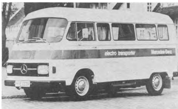
Fig. 3. Mercedes electric van. Battery type, lead-acid; rating, 144V, 150 A-hr; maximum range, 35 miles; maximum speed, 48 mph.
