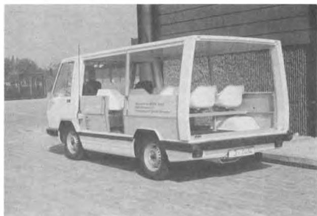
Fig. 1. The F.R.G. "marathon" van. Battery type, lead-acid; number of cells, 72; rating, 144V, 180 A-hr; maximum range, 65 miles; maximum speed, 50 mph; payload, 2200 lb.
