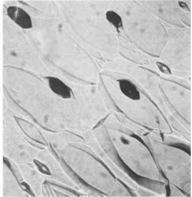
Fig. 4. Point-bottomed and deep pits produced along [110] direction on (001) face by mixture of H 2 SO 4 and H 2 O (1:3); etched for 5 min.
