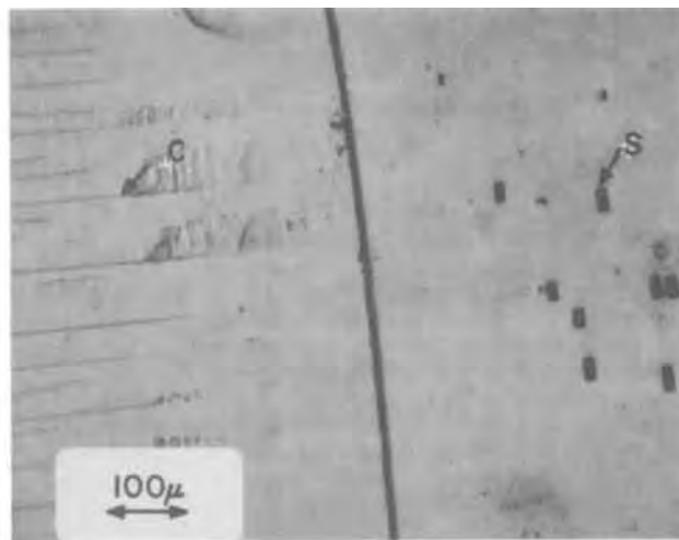
Fig. 6. InGaP/GaAs wafers which have been angle-lapped ( \sim 3^\circ ) to expose the GaAs substrate which exhibits rectangular etch figures (S) due to Sirtl etching. The InGaP portion exhibits cracks (c) due to (a) tension and (b) compression.
