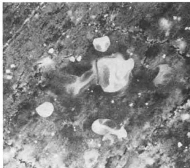
Fig. 11. Be electrode surface after polarization in 0.2M KI/DMF, H_2O = 0.3\% , V_i = 1.75 . Magnification 800X.
