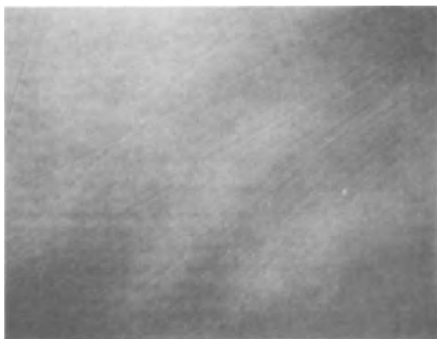
Fig. 2. "B" face of polished CdS wres viewed by Nomarski microscopy at 400X magnification. The "A" face is not shown because it is featureless under the same conditions of observation.
