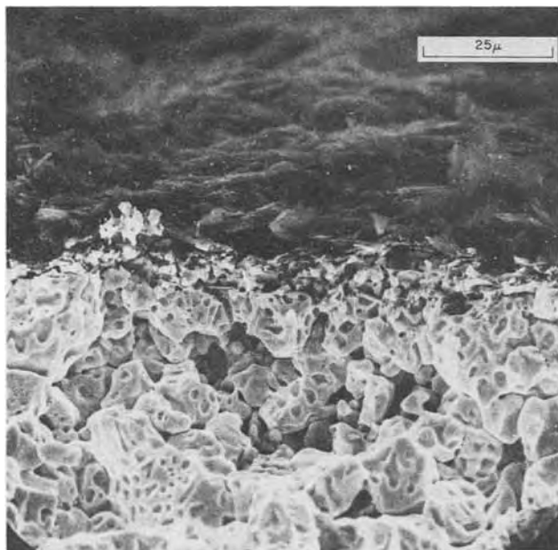
Fig. 8. Scanning electron micrograph of AgBr|C (pressed powder) interface after heating to 250°C.
