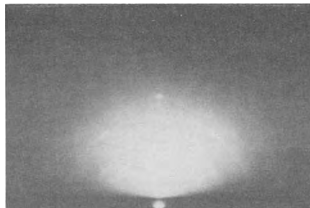
Fig. 6. Reflection electron diffraction pattern from a silicon surface which received Al diffusion, oxidation, and P diffusion heat-treatment. The surface is characterized by the presence of polycrystalline silicon and extra reflections resembling \eta\text{-Al}_2\text{O}_3 .
