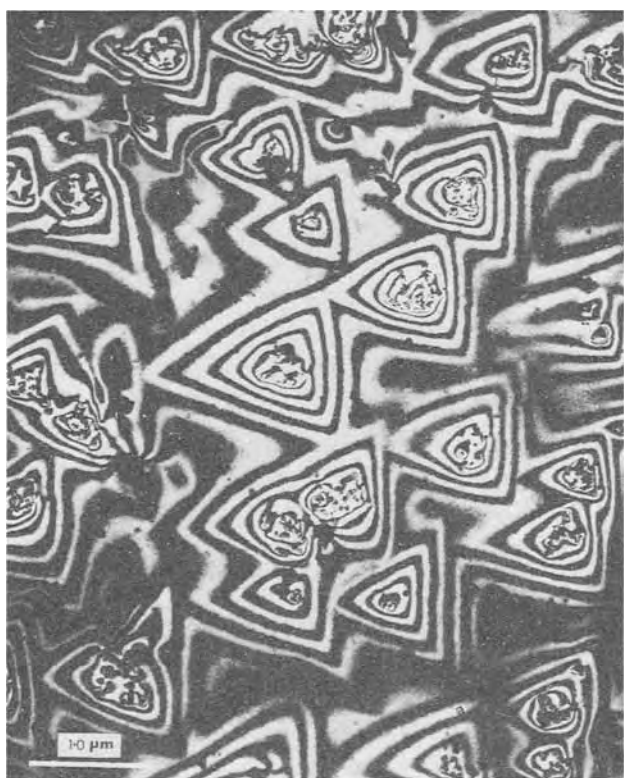
Fig. 7. \{220\} weak beam image of multiple fringes around precipitate clusters.
