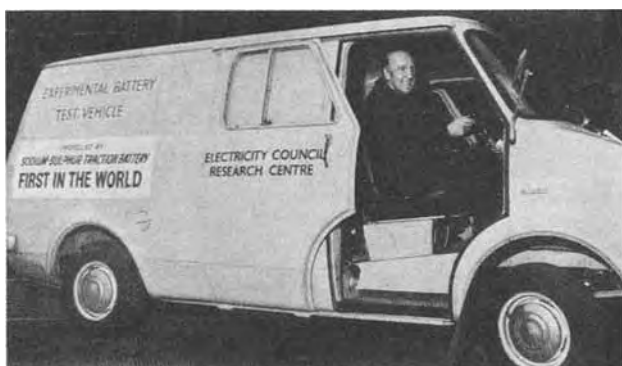
Fig. 11. Electricity Council Research Centre and British Railway sodium-sulfur powered electric vehicle.
