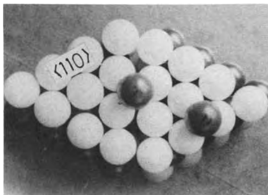
Fig. 4. Marble ball model of a noncoherent twin boundary. N, normal position; T, boundary position.
