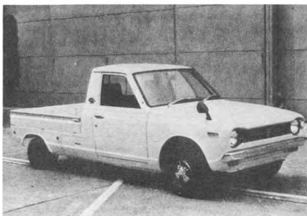
Fig. 10. Nissan short haul electric vehicle. Capacity, 96V, 125 A-hr; maximum range, 41 miles; maximum speed 32 mph; weight, 2000 lb; payload, 550 lb.
