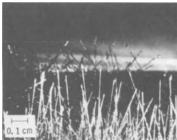
Fig. 1. Silicon whiskers growing from the inner walls of the alumina crucible at 1050°C in argon atmosphere.
