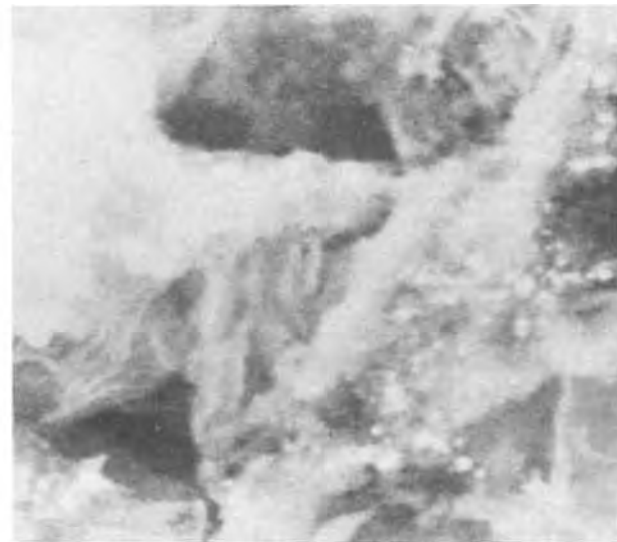
Fig. 12. Be anode polarized in 0.2M LiCl/MeOH, V_i = 0.34 , H_2O = 0.61\% . Magnification 2400X.
