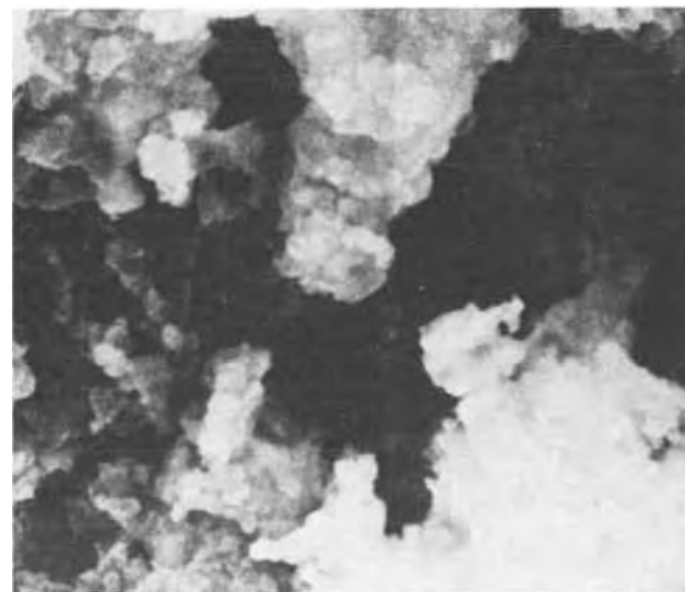
Fig. 9. Be anode polarized in 0.2M LiClO_4/EtOH at 24.5 \text{ mA/cm}^2 , H_2O = 0.4\% , V_i = 1.00 . Magnification 2400X.
