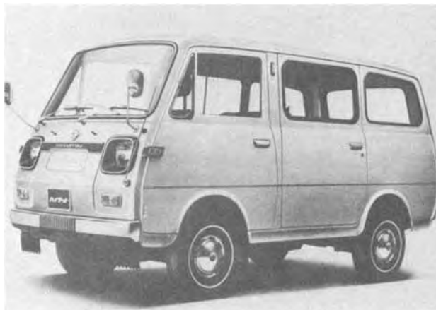
Fig. 9. Daihatsu S37 V-type electric van. Battery type, improved lead-acid; capacity, 72V, 125 A-hr; no. of batteries, 7; maximum range, 42 miles; maximum speed, 42 mph; weight, 1650 lb; payload, 550 lb.
