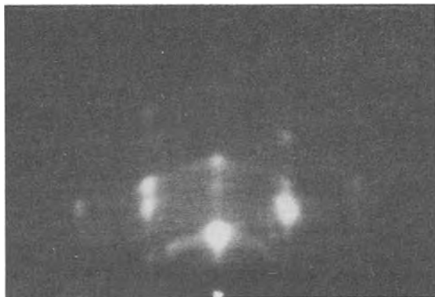
Fig. 4. Reflection electron diffraction from the surface of a silicon wafer following sealed tube Al diffusion indicating the presence of a faint ring pattern.
