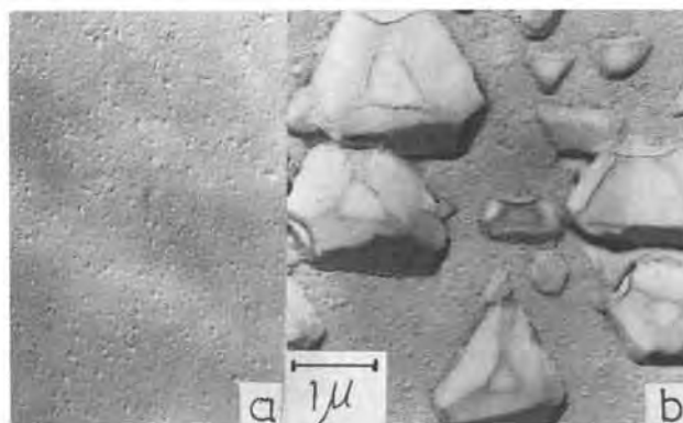
Fig. 11. Isolated nuclei on a mirror-smooth surface. Overpotential, 30 mV. a, Surface topography; b, trigonal pyramids.
